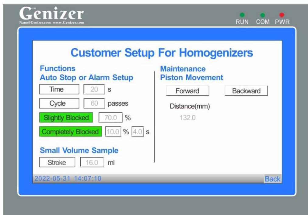
1) Time: set the timing and click "TIME" to start timing function, and then press the "START" button in the user operation interface to run the homogenizer. The equipment will stop automatically when the timing time is ended.
