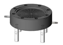
Install the four pillars (1) on the filter supporting base (2).
