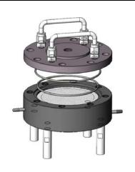
Install the small O-ring (4), large O-ring (5) and the gland (6) on the filter support base (2) in order.
